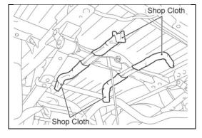
4. REMOVE THE PROTECTORS FROM THE SPARE TIRE CARRIER STOPPER
