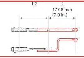
Connect the torque wrench to the Spare Tire Carrier Wrench so that they form a straight line when tightening.
