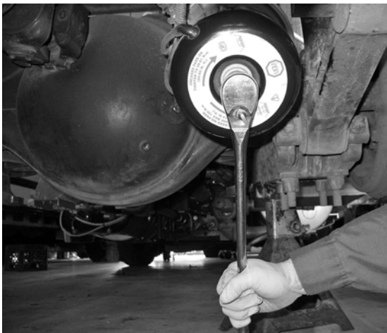
Figure 3. Caging Spring Brake Chamber
