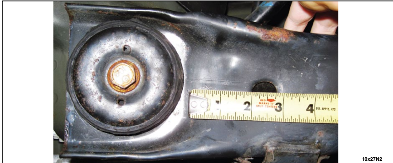
FIGURE 4 - Proper angle for a perforated subframe
