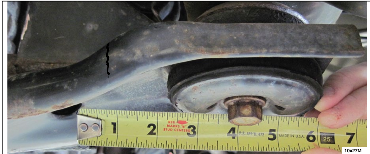
FIGURE 3 - Proper angle for a cracked subframe
