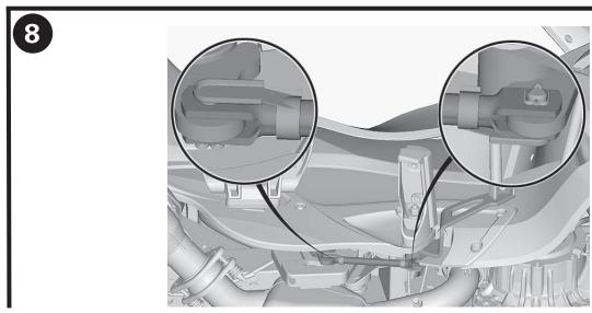
NEW RETAINING PINS PROPERLY INSTALLED
