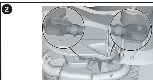
ORIGINAL RETAINING PINS TO BE REPLACED
