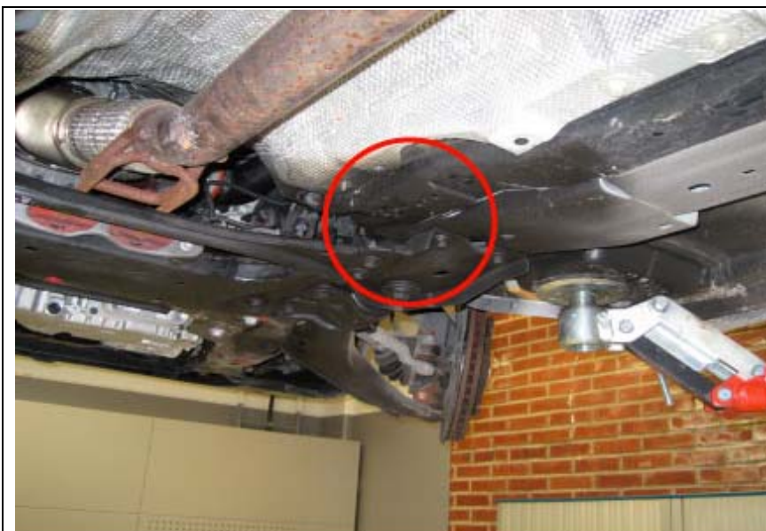
Location of conflict area under fuel rail.
