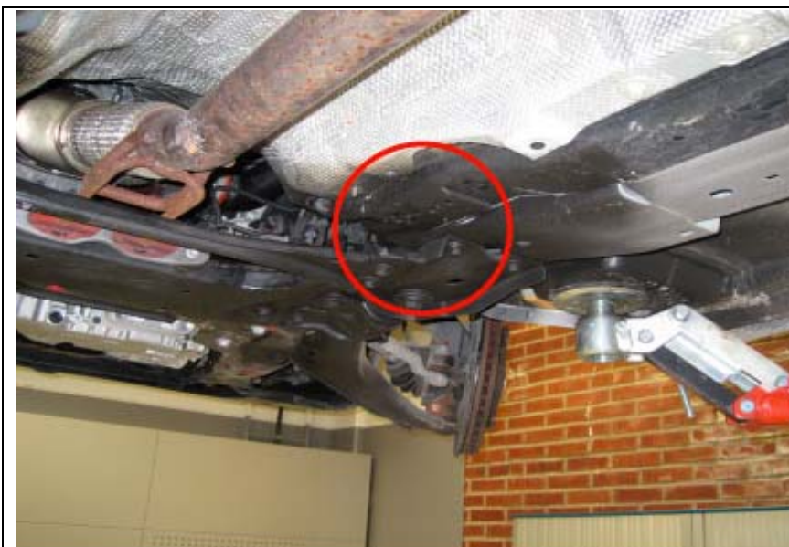
Location of conflict area under fuel rail.
