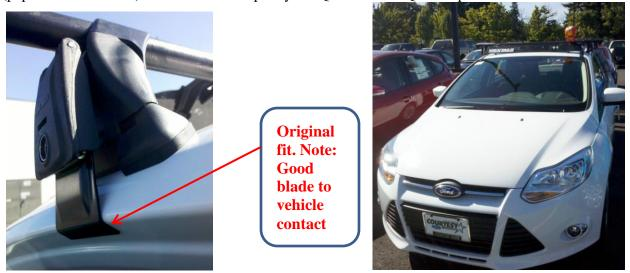
Note: Subsequent to the release, Yakima suspects that a modification to the Ford Focus (2012-2013 model year) door frame profile. This is supported by the pictures of the original fit versus the pictures of the fit on later production vehicles. This change causes the Yakima specified fit combination for this vehicle to be non-viable.
