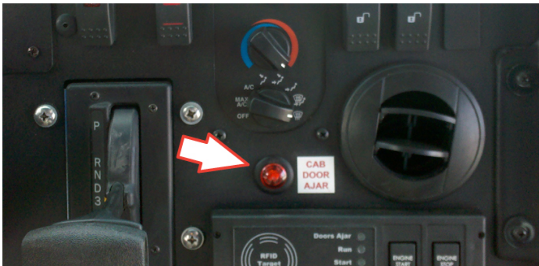
Door ajar light on dash panel (Freightliner shown)
