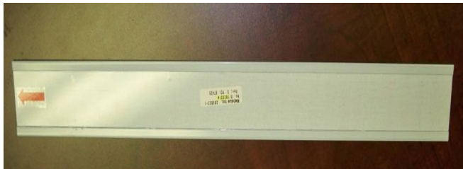
Figure 8 Interior part (side which will be glued) arrow pointing the corner molding.
