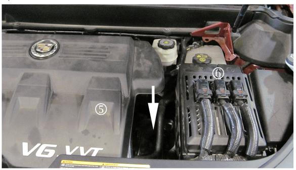
**Note:** Removal of the battery tray support is required to inspect or adjust the shift cable if the vehicle is equipped with turbocharger. Refer to *Battery Tray Support Replacement* in SI if the vehicle is equipped with a turbocharger.
