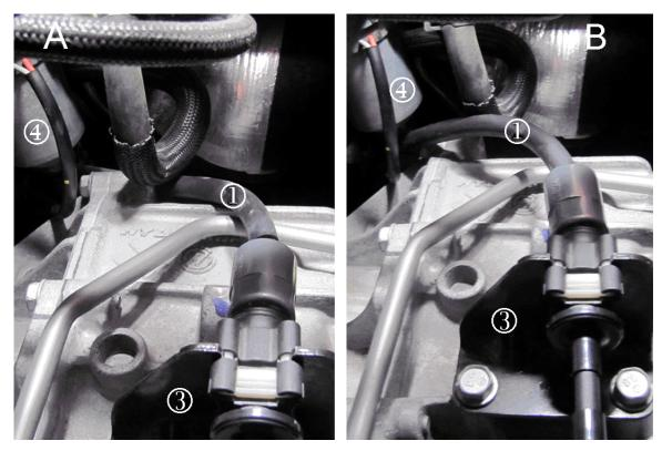
**Note:** Ensure that the transmission shift cable (1) is routed along the backside of the transmission and away from the power brake booster auxiliary pump (4). Refer to illustration. The "A" portion of the illustration shows a correctly routed transmission shift cable. The "B" portion of the illustration shows an incorrectly routed transmission shift cable.
