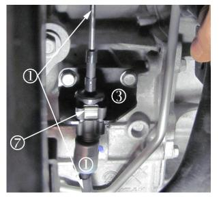
• If the transmission shift cable is NOT fully seated in the transmission cable bracket, install the transmission shift cable in the bracket, then slide the retainer (7) forward to lock the transmission range selector lever cable in the bracket. Pull up on the transmission shift cable to verify that the transmission shift cable is fully seated in the bracket. Proceed to step 5.
