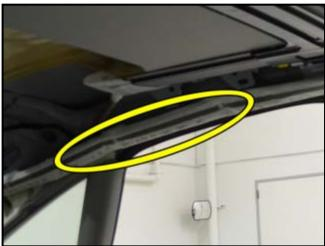
Warning: It is necessary that the "black line" <circle> be visible the entire length. By making sure it is visible the entire length will ensure that the head curtain airbag is NOT twisted
