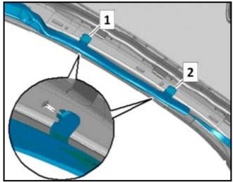
Remove the clips <1> and <2> from the A-pillar
