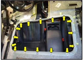
Tip: Picture on left shows location of 16 headliner clips <arrows> around sunroof frame
