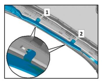
← Install the clips <1> and <2> in the Apillar and ensure that the "black line" is visible the entire length
