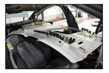
Note: Two technicians are needed to disconnect the last connections on the headliner. Be very careful when lowering the headliner as it bends easily
