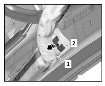
Carefully disengage the head curtain airbag <1> from each of the clips <2> <arrow>
