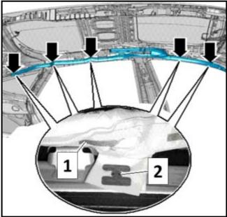
Remove the clips <arrows> from the head curtain airbag <1> with pliers
