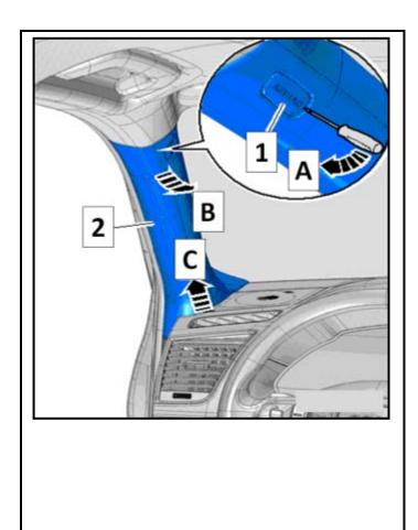
← Pry out the expanding cap <1> with the "AIRBAG" symbol about 4mm with a screwdriver <arrow A>
