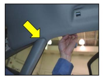
← Lift the headliner carefully over the remaining C-pillar trim <arrow>
