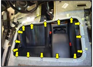
Tip: Picture on left shows location of 16 headliner clips <arrows> around sunroof frame
