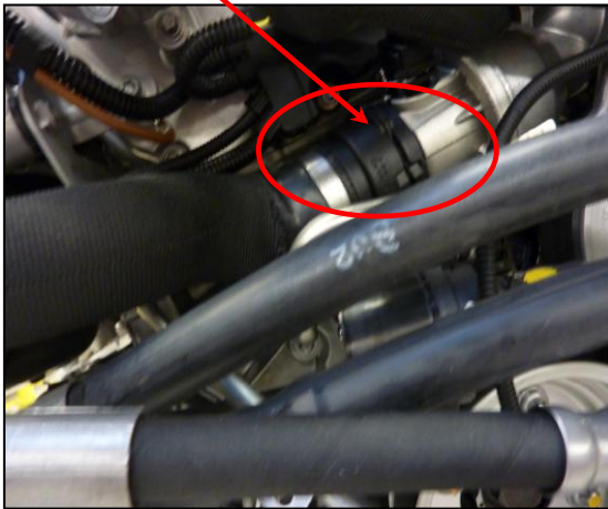
Figure 2, above left, shows the lower coolant hose fitted.
