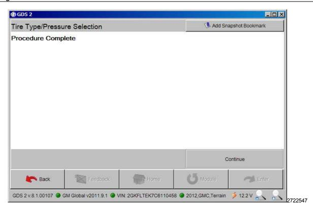
2.12 After the Procedure Complete message appears on the Tire Type/Pressure screen, exit GDS2.
