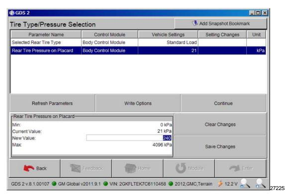
2.8 Select Rear Tire Pressure on Placard from the Tire Type/Pressure Selection screen.
