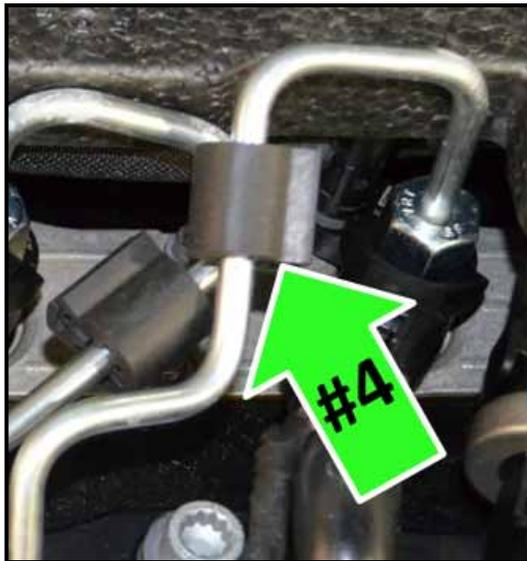
⇐ Install fuel line dampener (03L 130 118) in the center of #4 fuel line as shown <arrow>
