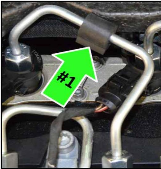
⇐ Install fuel line Damper (03L 130 118) in the center of #1 fuel line as shown <arrow>
