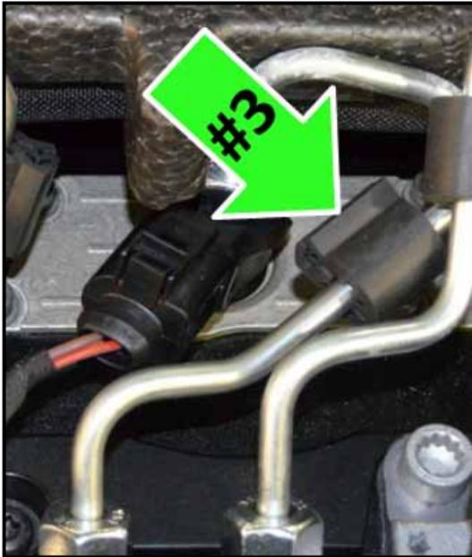
⇐ Install fuel line Damper (03L 130 118) in the center of #3 fuel line as shown <arrow>
