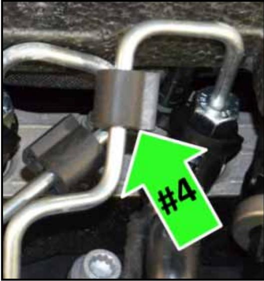
⇐ Install fuel line Damper (03L 130 118) in the center of #4 fuel line as shown <arrow>
