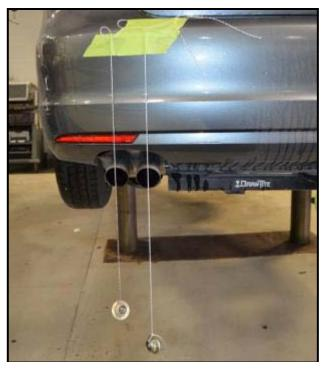
Section D – New Exhaust Tip Installation (Criteria 02, 03 vehicles ONLY)
