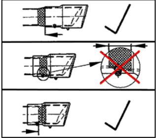
Note: Ensure that screws are NOT positioned over flared portion of exhaust (see drawing on left).
