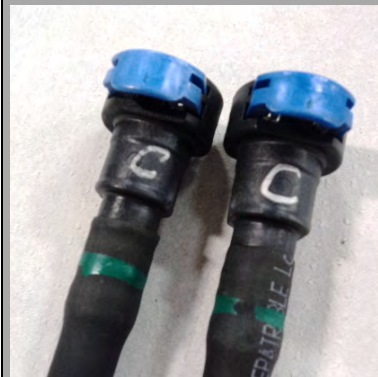
Replacement fuel lines
