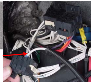
Fig. 5—12 ga. wire installed in gray plug.
