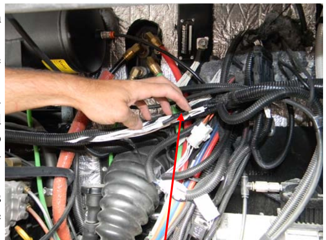
Fig. 15— Front cap harness #38110513—wire splice.
