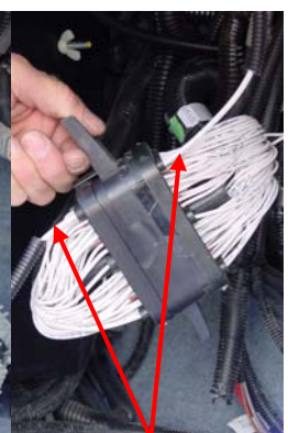
Fig. 10—12 ga. wiring installed in connector.
