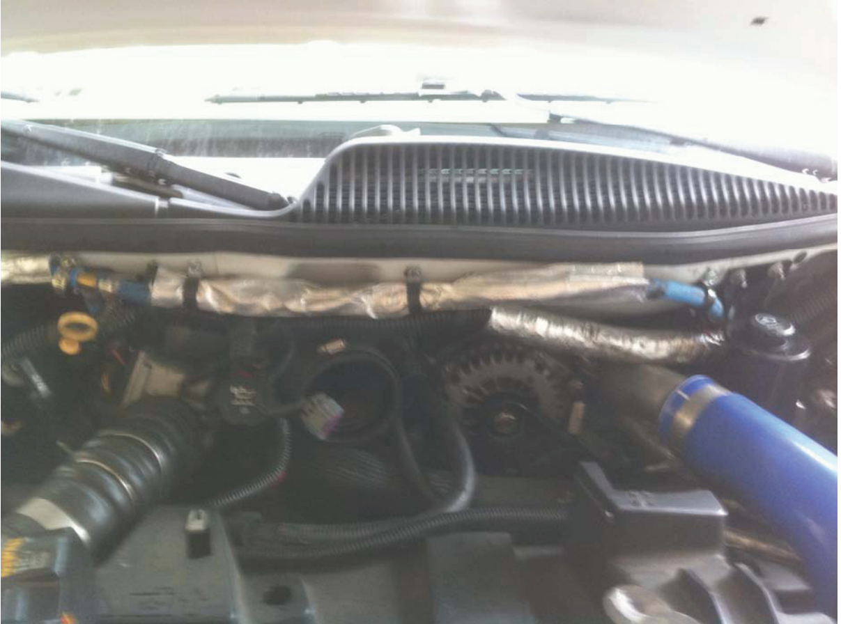
Picture 6 is a full under hood view of the hoses rerouted and p-clamped in place.
