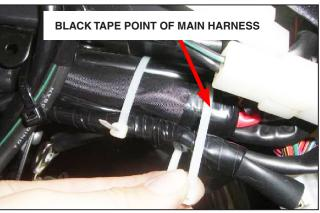
18. Fasten point 5 – Using a short cable tie (145mm) from the kit, combine the wire sub-lead with the main harness at the white tape point of the wire sub-lead. Face the end of the cable tie forward. Do not cut off the end of the cable tie.
