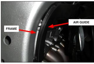
7. Route the wire sub-lead between frame and air guide. Then route the wire sub-lead along the main harness.
