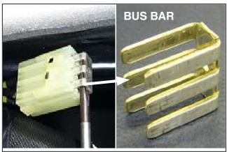
4. If the ground joint connector is damaged, the entire wire harness itself must be replaced.
