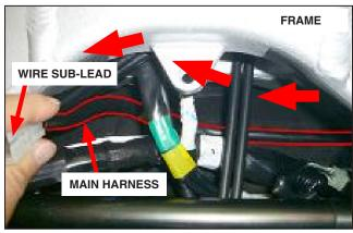
12. Connect the wire sub-lead to the ground joint connector where the connector cover and bus bar were removed.
