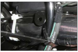
17. Fasten point 4 – Using a short cable tie (145mm) from the kit, combine the wire sub-lead with the main harness at the black tape point of the main harness. Face the end of the cable tie outward. Do not cut off the end of the cable tie.
