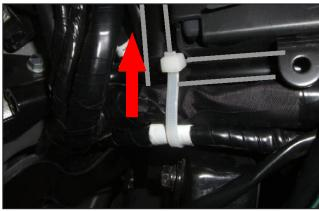
15. Fasten point 2 – Using the medium cable tie (202mm) from the kit, combine the wire sub-lead with main harness, right radiator fan motor lead, negative battery lead, and starter motor lead. Face the end of the cable tie outward. Position the cable tie in front of the air deflector. Make sure the cable tie is on the fan motor lead's protective sleeve, and then cut off the excess end of the cable tie.
