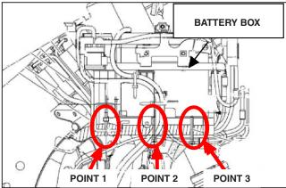
14. Fasten point 1 – Using the long cable tie (383mm) from the kit, combine the wire sub-lead with the main harness and stay 1 at the white tape point of the wire sub-lead. Face the end of the cable tie upward as shown, and then cut off the excess end of the cable tie.
