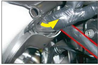
11. Route the wire sub-lead along the main harness from right side to left side.
