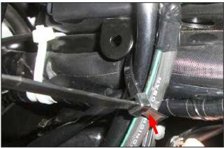
16. Fasten point 3 – Using a short cable tie (145mm) from the kit, combine the wire sub-lead with main harness, right horn lead, right radiator fan motor lead, and stay 1 at the original point. Face the end of the cable tie outward. Make sure to install the cable tie on the fan motor lead's protective sleeve. Do not cut off the end of the cable tie.
