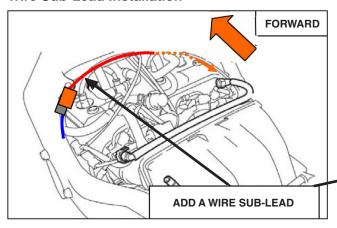
Locate the negative lead coupler under the battery.
