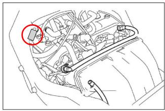
To correct this defect, Yamaha is initiating a Factory Modification Campaign. Affected motorcycles must have an additional wire sub-lead installed or, if the ground joint connector has already been damaged from overheating, have the main wire harness replaced.
