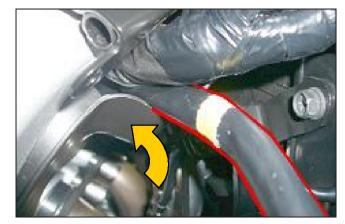
10. Route the wire sub-lead behind the main harness as shown.
