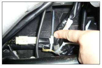
19. Fasten point 6 – Using the last short cable tie (145mm) from the kit, combine the wire sub-lead with main harness by the white tape point of the wire sub-lead at point 6. Face the end of the cable tie forward. Do not cut off the end of the cable tie.
