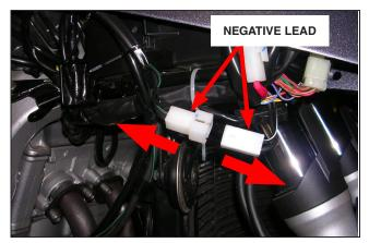
3. Connect the wire sub-lead couplers to the negative lead couplers.
