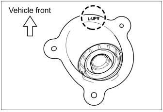
b) Check the orientation before installing the new dust
