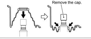
2) Position the dust seal on the shaft correctly.
