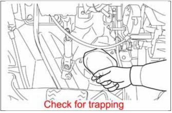
c) Install the new dust seal.
