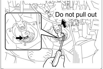
c) Use a flathead screwdriver wrapped in tape to lift the intermediate shaft so that the pinion shaft is visible.
