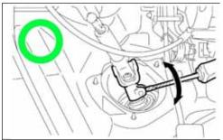
If the shaft is stuck, insert a flathead screwdriver wrapped in tape into the slit and pry.
