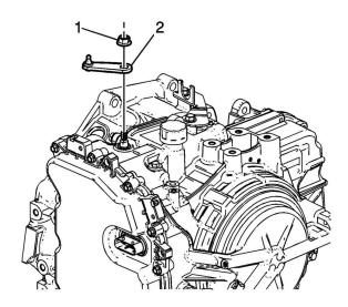
Warning: The transmission shift lever terminal end MUST be disconnected from the transmission manual shaft lever BEFORE the securing nut is removed. Attempting to loosen the manual shaft lever securing nut with the transmission cable still attached may internally damage the cable, creating a binding condition that will necessitate transmission cable replacement.
