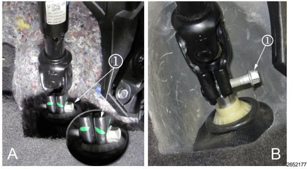
(A) Lower Intermediate Steering Shaft Bolt Fully Seated(B) Lower Intermediate Steering Shaft Bolt NOT Seated(1) Lower Intermediate Steering Shaft Bolt.
