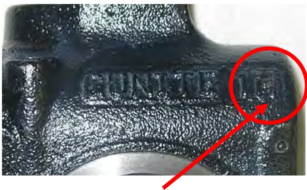
Figure A: Mold Line Nomenclature
