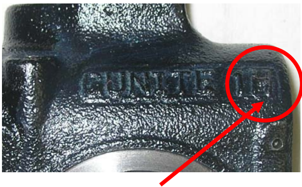
Figure A: Mold Line Nomenclature
