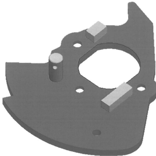
Fig. 9 Top and Bottom views of the new cams 50726261 and 50726261-01 (Used for modification of teeter lever assembly 50530211-04 - with resilient lock)
