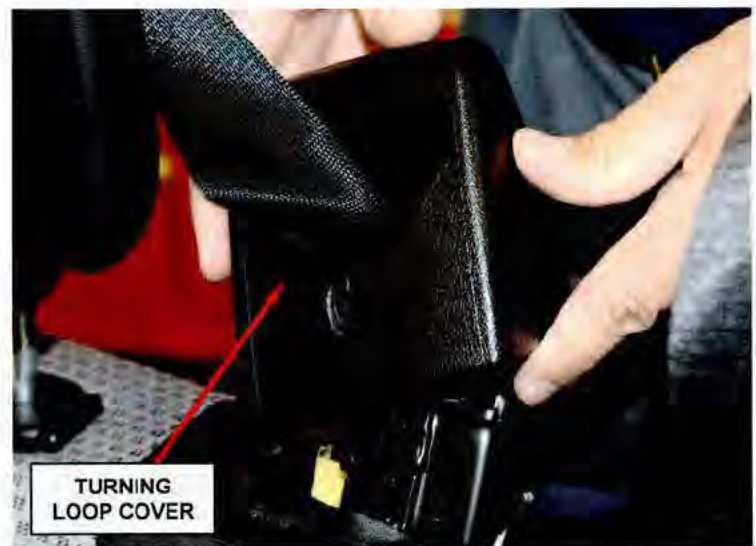
Figure 9 – Install Seatbelt Turning Loop Cover
