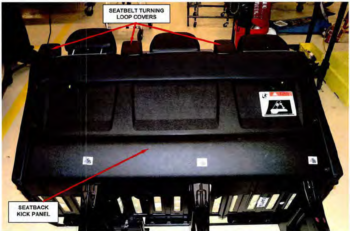
Figure 2 – Seatback Kick Panel and Seatbelt Turning Loop Covers
