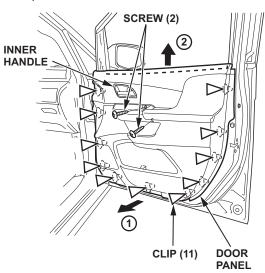
6. While holding the door panel away from the door, remove the inner handle from the door panel by releasing the hooks.
