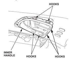
7. Remove the door panel while pulling out the inner handle through the hole in the door panel. While holding the door panel away from the door, disconnect the courtesy light connector.
