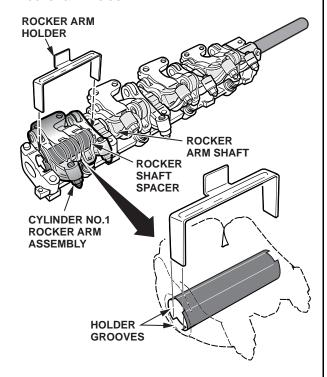
Remove the cylinder No. 1 rocker arm assembly from the rocker bridge assembly.
