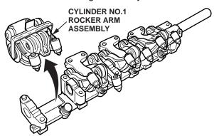
11. Repeat step 10 for the remaining three rocker arm assemblies. Note the location of each assembly to make sure they are returned to their original positions.
