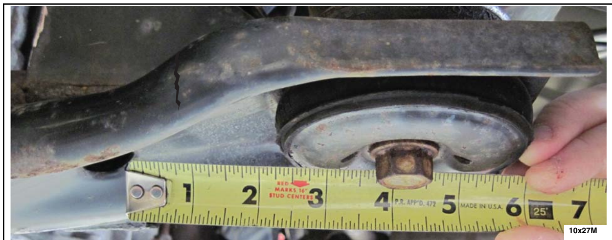
FIGURE 3 - Proper angle for a cracked subframe
