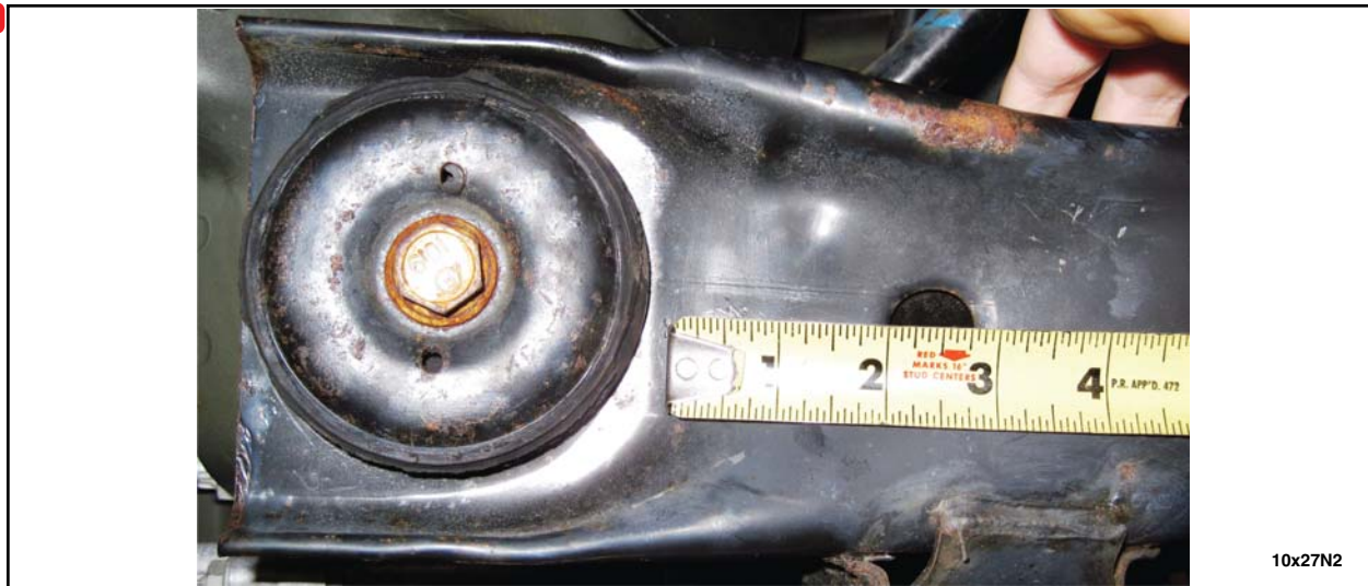
FIGURE 4 - Proper angle for a perforated subframe
