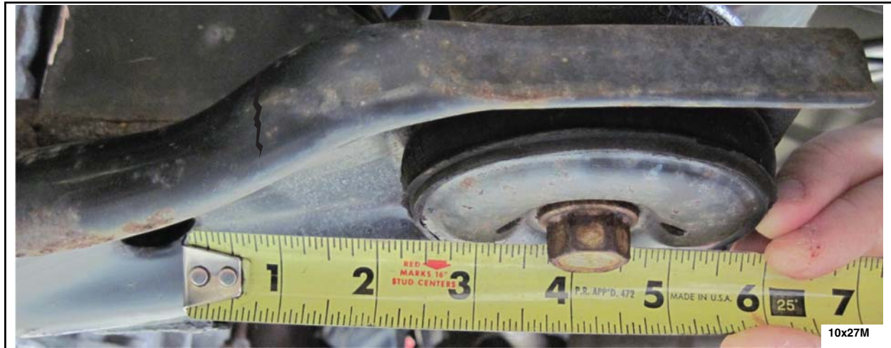
FIGURE 3 - Proper angle for a cracked subframe
