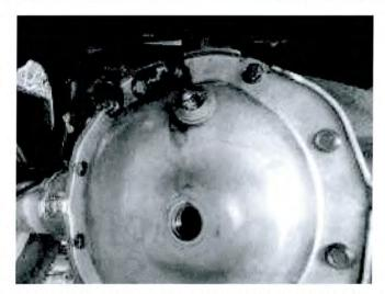
17. Remove the fill plug using a ratchet with a 3/8" extension and a 1/2" square head.
