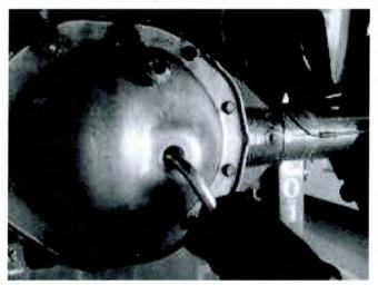
18. Fill the axle with 2 litres (2.1 quarts) of new oil. Verify the fluid level after filling the oil to be less than 2 cm (0.79 in) below the fill hole.
