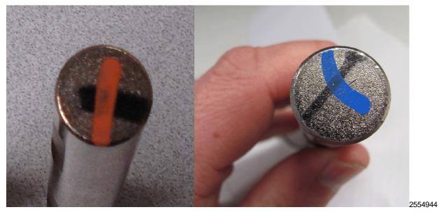
Note: If **BOTH** lines are not clearly visible on the cross pin, the cross pin MUST be replaced.
