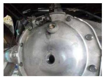
17. Remove the fill plug using a ratchet with a 3/8" extension and a 1/2" square head.
