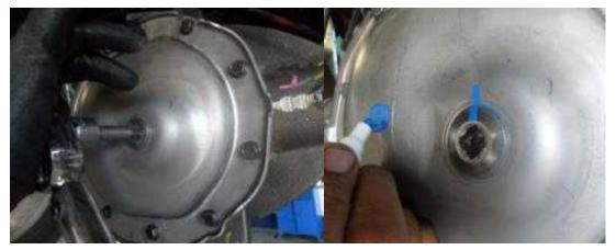
19. Reinstall the original fill plug, hand start it and apply a static torque of 35 Nm (26 lb-ft) with a pre-set clicker wrench.
