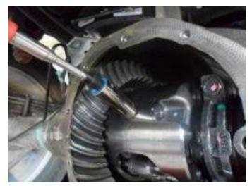
12. Using a magnet, insert a new certified cross pin without moving the case position, aligning the cross pin hole with the lock screw hole.
