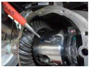
11. Remove the cross pin by pulling it with the magnet. Discard the cross pin.
