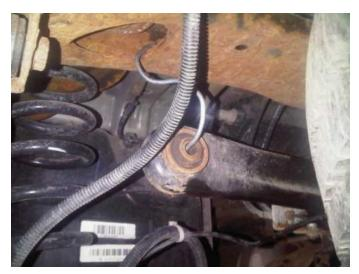
5. FOR SUV ONLY: Raise the track bar, hanging it with a hook to the frame.
