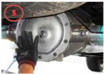
6. Take the cover pan bolts off using a ratchet with a 13 mm socket. Hold the cover pan with your hand to drain the oil in a container. Retain the cover pan bolts.
