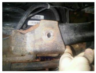
21. FOR SUV ONLY: Unhook the track bar from the frame making sure to remove the hook from the vehicle. By applying a lateral push on the wheel, align the track bar hole to the axle. Hand start the track bar bolt and apply a static torque of 105 Nm (77 lb-ft) with a preset clicker wrench.
