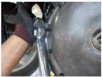
**Note:** Reuse cover pan bolts. Ensure that the bolts have been cleaned before they are installed. Apply Loctite 272 or equivalent to the threads of the cover pan bolts.
