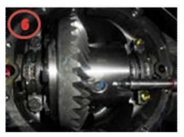
10. Remove the lock screw with a ratchet with a 5/16" hexagonal socket while holding the cross pin with a magnet. Dispose of the lock screw.
