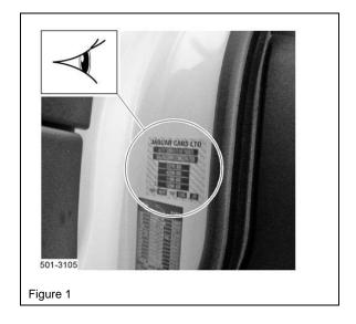
NOTE: Verify that the VIN on the replacement label matches the VIN in the lower left of the front windshield.
