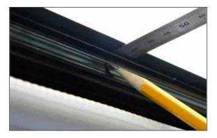
Measure the length of the urethane bead between the marks. The length of each bead must be at least 40mm. Repeat the step for the other five urethane beads.
