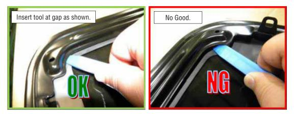
**NOTE:** If the moonroof passes both the Urethane Bead Inspection Procedure and the Moonroof Glass Corner Separation Test, then no further action or repair is required.
