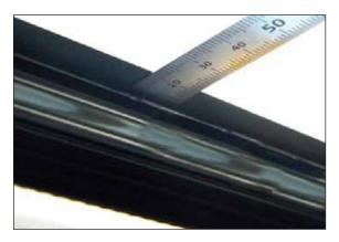
Slide the ruler between the moonroof glass and moonroof frame. Slide the ruler in a sideways motion until you locate one of the ends of the urethane bead. Using a pencil, place a small mark on the frame to mark the position.
