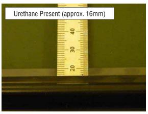
Slide the ruler along the bead until you can locate the other end of the urethane bead. Place a small mark on the frame to mark that position.
