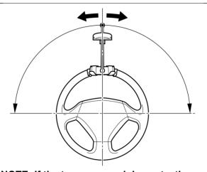
NOTE: If the torque wrench is contacting the windshield or A-pillar when taking this measurement, the attachment position can be moved to another spot on the circumference of the steering wheel.
