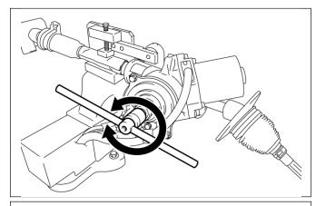
b) Set the pinion shaft by performing the following a total of 3 times: Rotate the shaft 1 rotation right of center then 1 rotation left of center.
