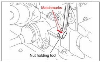
c) With the adjusting nut held by the holding tool, add match marks to the tool and gear.
