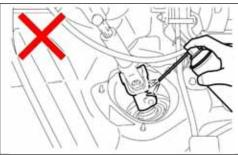
NEVER apply lubricant to the shaft. Doing so will change the friction coefficient, and may cause the bolt to become loose or to break when tightened.
