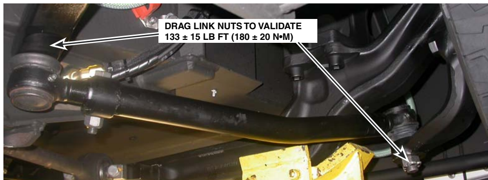
Figure 1 - Steering drag link
