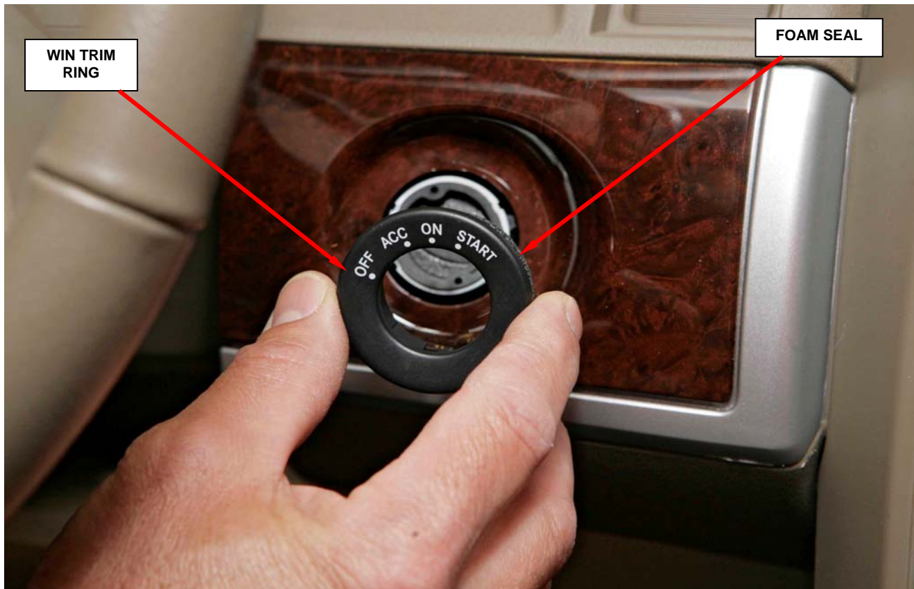
Figure 4 – Install WIN Trim Ring with Foam Seal
