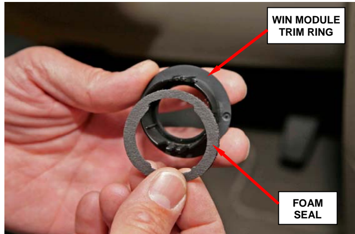
Figure 3 – Install Foam Seal
