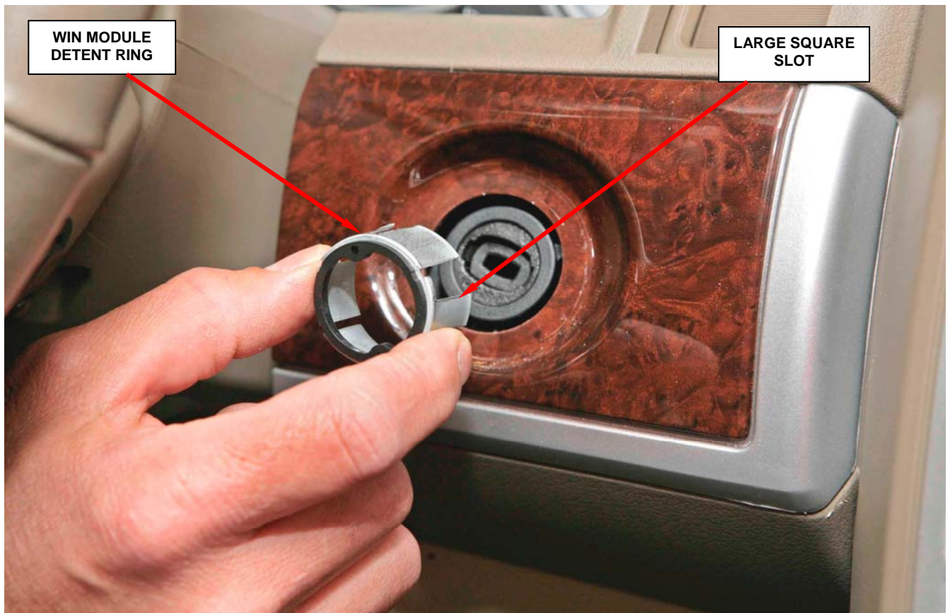
Figure 2 – Install WIN Module Detent Ring
