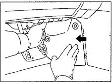
4. REINSTALL THE ACCELERATOR PEDAL ASSEMBLY
