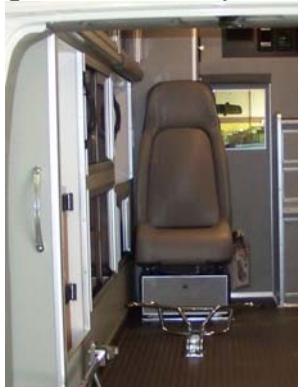
Before: Child Safety Seat on steel base with Type 1 seat belt assembly
