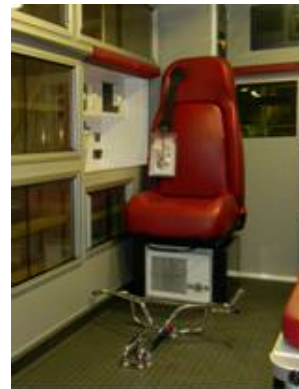
After: Child Safety Seat on steel base with Type 2 seat belt assembly
