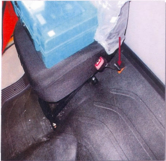
View of suspect RH inboard seat belt anchor location
