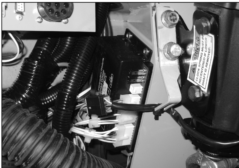
Figure 11. Reference photo of VIP controller.
