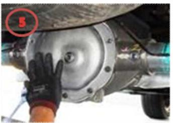
6. Take the cover pan bolts off using a ratchet with a 13 mm socket. Hold the cover pan with your hand to drain the oil in a container. Dispose of the bolts.
