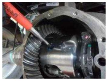
10. Remove the cross pin by pulling it with the magnet. Discard the cross pin.
