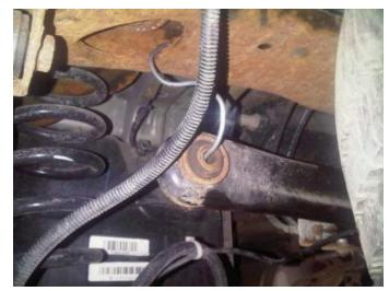
5. FOR SUV ONLY: Raise the track bar, hanging it with a hook to the frame.
