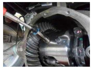
11. Using a magnet, insert a new certified cross pin without moving the case position, aligning the cross pin hole with the lock screw hole.
