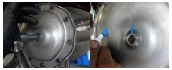
18. Reinstall the original fill plug, hand start it and apply a static torque of 35 Nm (26 lb-ft) with a pre-set clicker wrench. Certify, applying a slash through the fill plug and the cover pan.
