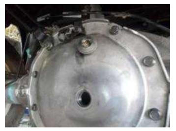
16. Remove the fill plug using a ratchet with a  $3/8^{\circ}$  extension and a  $1/2^{\circ}$  square head.
