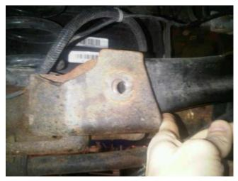
20. FOR SUV ONLY: Unhook the track bar from the frame making sure to remove the hook from the vehicle. By applying a lateral push on the wheel, align the track bar hole to the axle. Hand start the track bar bolt and apply a static torque of 105 Nm (77 lb-ft) with a preset clicker wrench.
