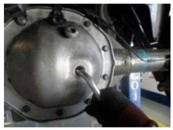
17. Fill the axle with 2 liters (2.1 quarts) of new oil. Verify the fluid level after filling the oil to be less than 2 cm (0.79 in) below the fill hole.
