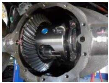
7. When most of the oil is drained, remove cover pan and gasket. Store the cover pan and gasket in a secure area.
