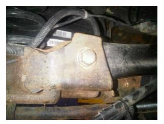
3. FOR SUV ONLY: Remove the LH track bar attachment bolt using a 21 mm socket.
