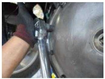
**Note:** Replace 9 out of the 10 cover pan bolts. Reuse cover pan bolt attached to the bracket. Apply Loctite 242 or equivalent to the threads of the cover pan bolt attached to the bracket.
