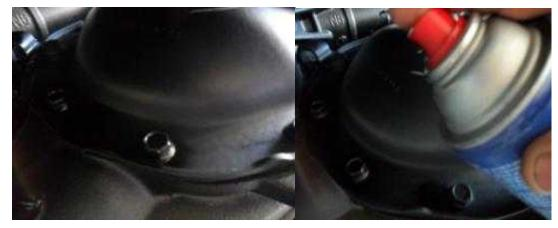
19. Clean the axle surface from oil residuals using a multipurpose solvent and clean towel. Spray black paint over the bolt heads and fill plug.
