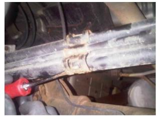
4. FOR SUV ONLY: Remove with a screwdriver the emergency brake cable clip from the track bar.
