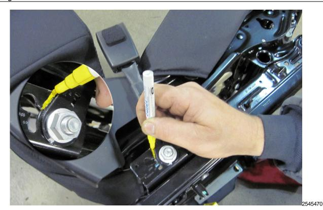
**Note:** The seat belt buckle assembly angle must be marked with a marker prior to removal so that the seat belt buckle assembly alignment is correct on reassembly.
