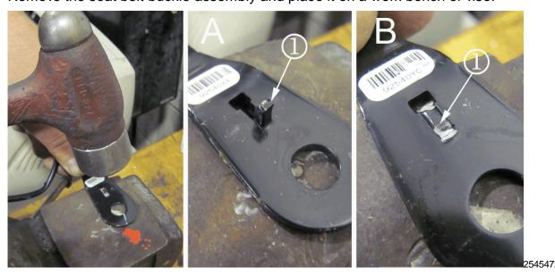
5. Using a hammer, bend the anti-rotation tab (1) on the seat belt buckle assembly. Ensure that the anti-rotation tab is bent down into the tab notch (B). Refer to the illustration.
