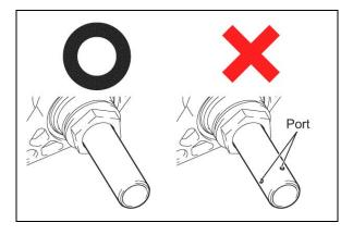
e) Confirm that the piston ports are in the correct position as shown.
