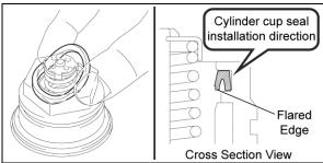
b) Install the **NEW** rubber seal (brake master cylinder cup) by hand, making sure the flared edge is facing down.
