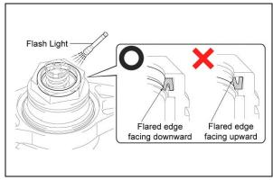
c) Confirm the positioning of the **NEW** rubber seal (brake master cylinder cup), making sure the flared edge is facing down.
