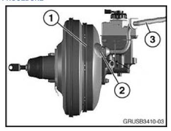
1. Remove the brake booster vacuum supply line (3) together with the non-return valve (2) from the brake booster (1).
