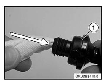
2. Check the brake booster vacuum supply line at the non-return valve upstream from the brake booster for contamination of oil. Insert a tightly rolled up corner of a non-reusable lint free white shop towel (see arrow) into the non-return valve (2). If the towel does not indicate any engine oil residue, proceed to step 4.
